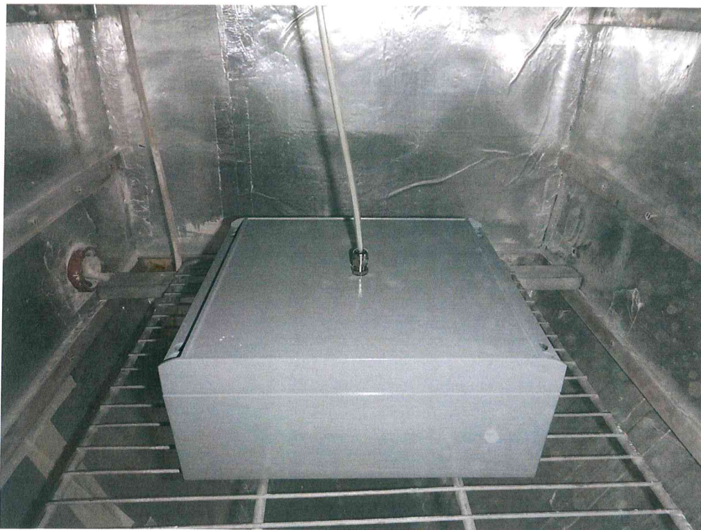
Figure 1 Exposition IP Code 6X
