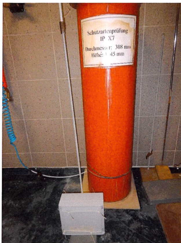
Figure 3 Exposition IP Code X7
