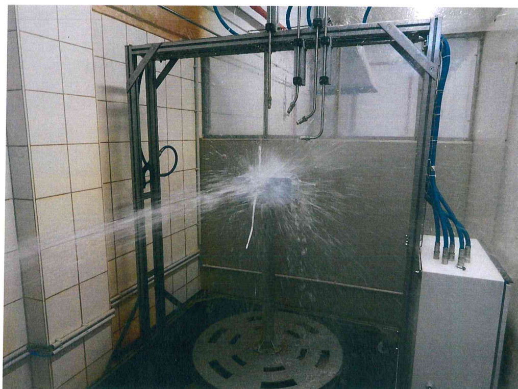
Figure 2 Exposition IP Code X6
