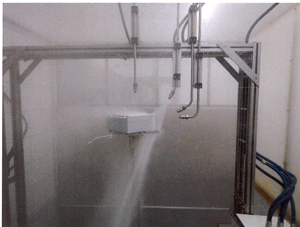
Figure 4 Exposition IP Code X9K, 60°, example
